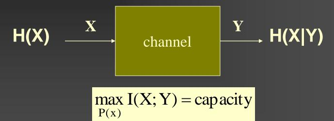
notes: capacity depends on input probabilities because the transition probabilites are fixed
