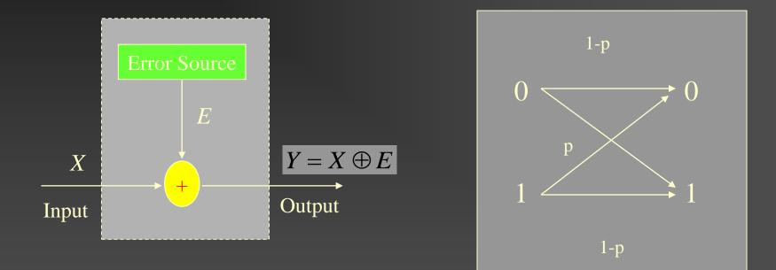
E is the binary error sequence s.t. P(1) = 1-P(0) = p X is the binary information sequence Y is the binary output sequence
